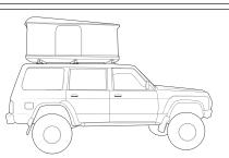
When these roof racks are to be used on a vehicle that is driven off sealed roads, the manufacturer maximum roof load rating (to be found in the vehicles User Manual) should be *divided by a factor* of 1.5. Do not forget to subtract 5kg from your maximum carrying capacity due to the weight of the crossbars and legs.
