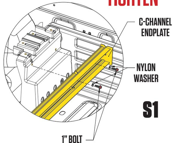
**RECOMMENDED TORQUE:** Bolts in S1 and S2 BAG - 27 in-lb. / 3Nm.
