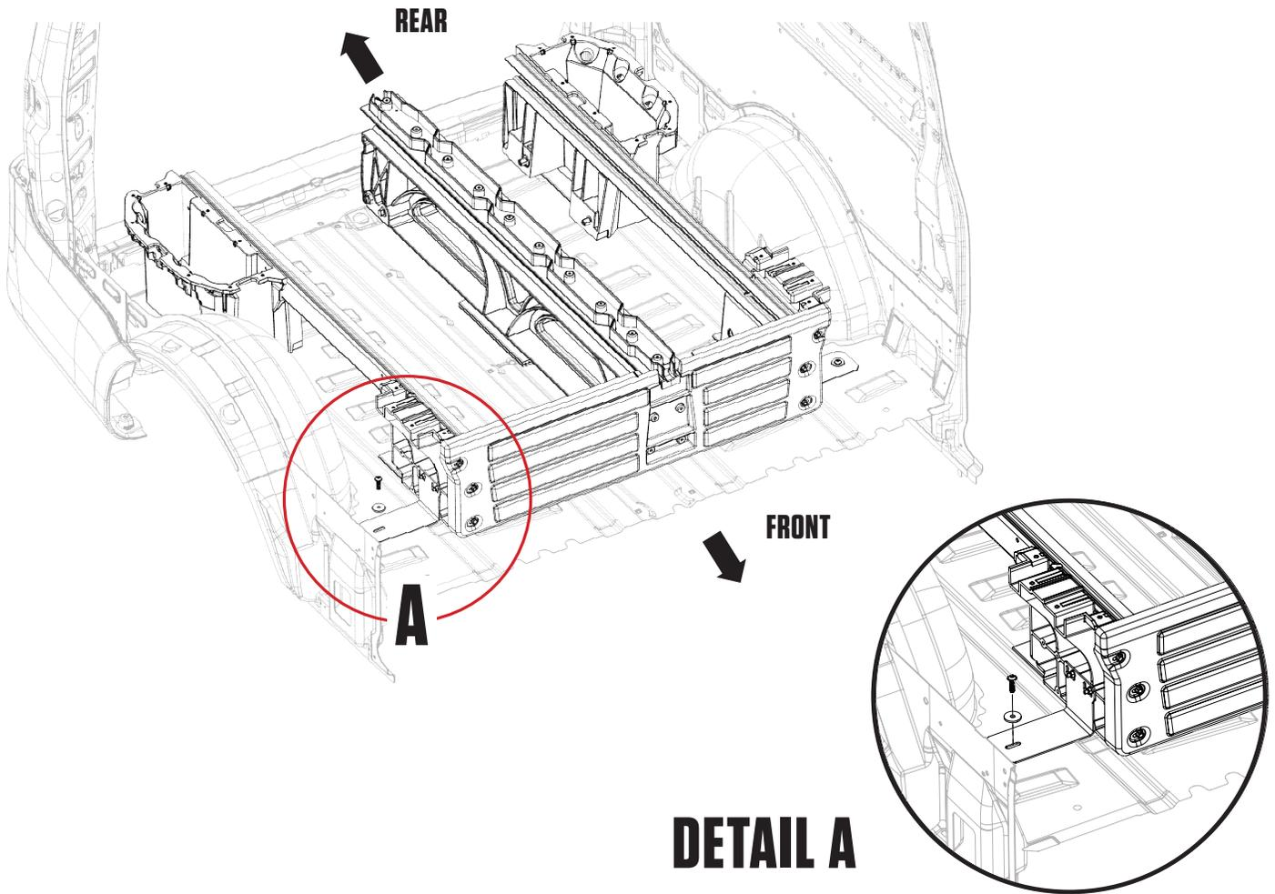
**RECOMMENDED TORQUE: Bolts in PREP METVIT BAG - 27 in-lb. / 3Nm.**
