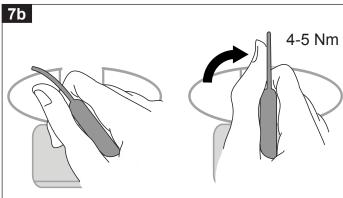
With Torque Key inserted (Item 7), turn clockwise until handle straightens out as shown above. This indicates 4-5 Nm. More pressure may be required in extreme climates.
